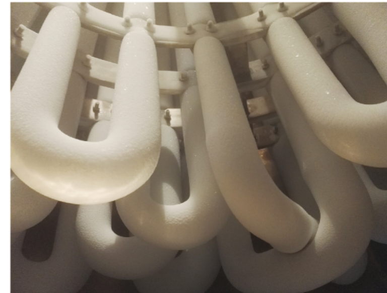
Ice-capture Picture in AUSTAR Freeze Dryer
